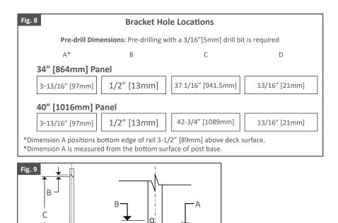
• It's important to double check dimensions to confirm accuracy of bracket hole locations before drilling.
