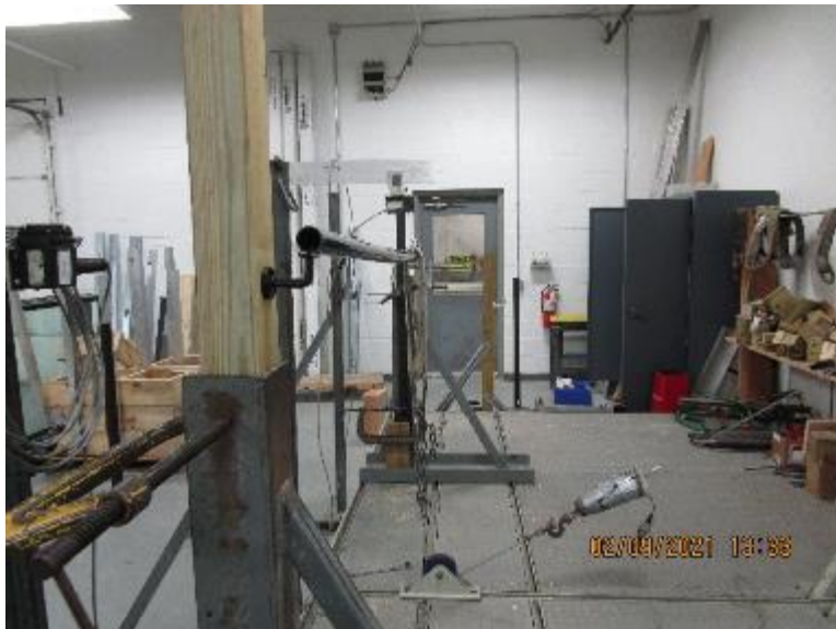
Photo No. 6 Concentrated Vertical Load Test at Mid Span
