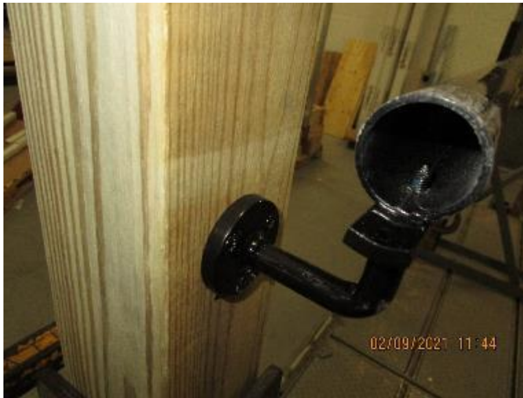
Photo No. 3 Bracket Connection - 4x4
