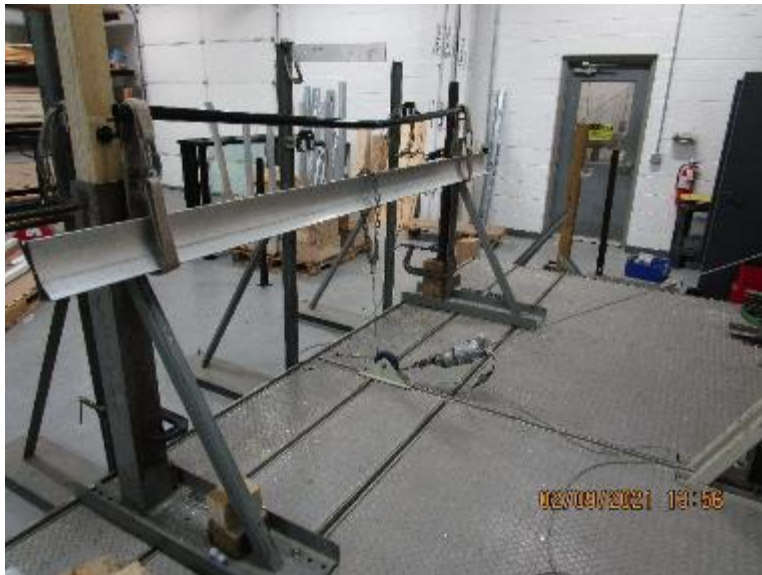
Photo No. 8 Concentrated Vertical Load at Brackets
