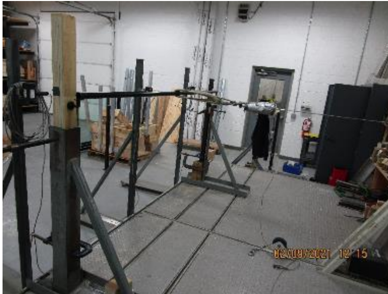
Photo No. 5 Concentrated Horizontal Load Test at Mid Span
