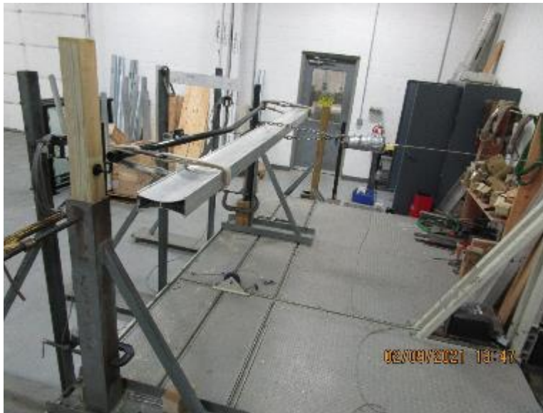
Photo No. 7 Concentrated Horizontal Load at Brackets
